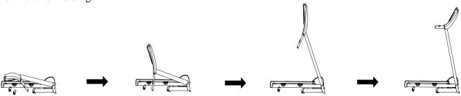
**STEP 2:** According to the picture to tighten the bolt M8\*45 (D16), M8\*15 (D13) and inner washer (D17). Then Locked with M8\*15(D13) and inner washer (D17).
